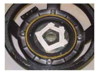
• Clean the magnet air gap using double face adhesive tape, then tape over the gap to keep any dirt from entering.
