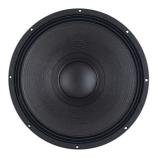
The new B&C 18RBX100 anchors our ferrite subwoofer line, and features an all new FEA optimized motor structure. The 25mm high, 4" (100mm) diameter copper wire voice coil is combined with a laminated double silicone spider, water resistant curvilinear cone and triple roll surround, for even more excursion and linearity.
